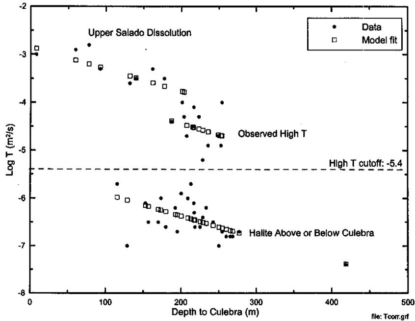
Figure 12. Correlation between Culebra T and overburden thickness for different geologic environments.
